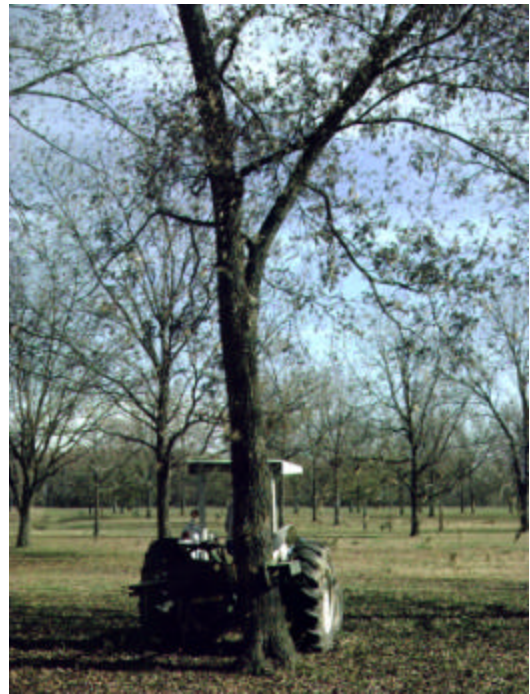
A PTO driven hydraulic tree shaker facilitates the prompt harvest of pecans
