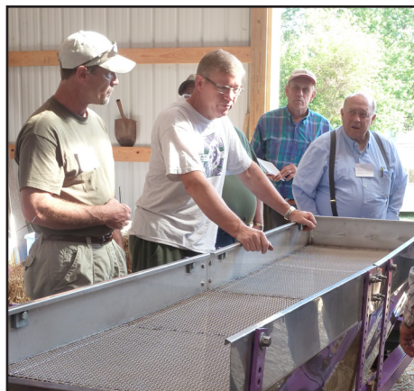
Darrel Durham demonstrates how to operate a second-generation prototype machine that will mechanically de-stem elderberry fruit
