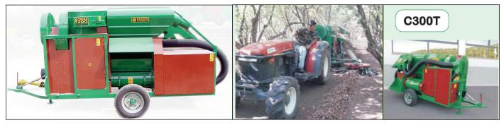
The C300T mechanical vacuum harvester hard at work. When used by chestnut growers, it can sweep and vacuum in over 1,300 pounds of chestnuts per hour. This harvester also removes the spiny bur from each chestnut, and can help minimize labor costs for chestnut growers. Photos courtesy of FACMA.
