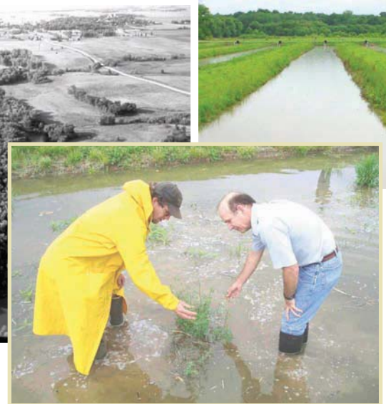
Top Left: Aerial view, Missouri River bottomland area. Top Right: The 12 channels of the HARC flood laboratory can be independently controlled for water flow. Bottom: Researchers evaluate hardwood seedlings planted in a flood laboratory channel.
