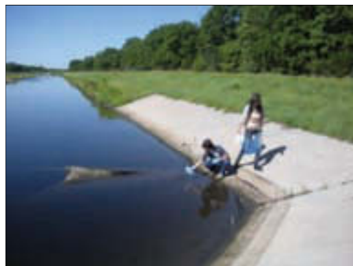
Collecting water samples at a constructed wetland connected to a wastewater treatment plant to evaluate effectiveness of wetlands in removing pharmaceuticals & personal care products.
