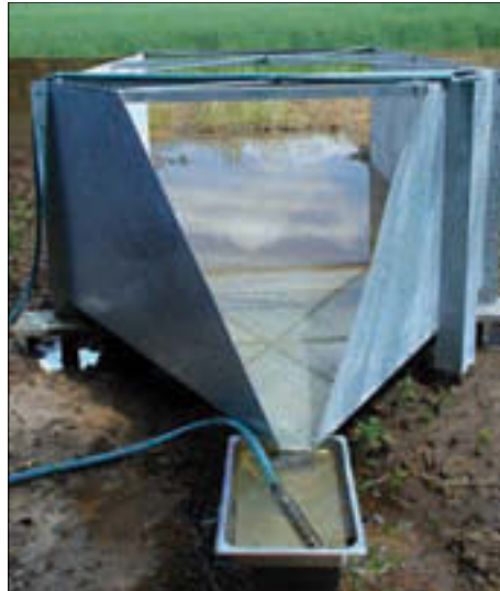
A flume is installed at a field edge to collect and measure runoff.
