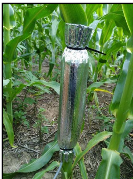
Fig. 2. Corn plant with the insulation cover to protect the sensor..
