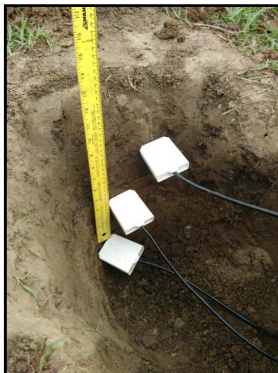
Fig. 3. Soil moisture sensors at 5 cm, 10 cm, 20 cm and 40 cm soil depths.
