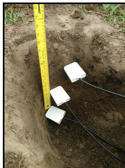
Fig. 3. Soil water reflectometers installed at 10 cm, 20 cm, 30 cm depths.
