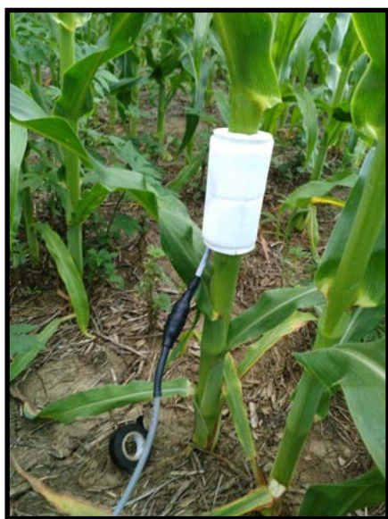
Fig. 1. Corn plant with a sensor with a wire that connects to a data logger.
