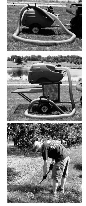
Fig. 1. Harvest equipment evaluated for harvesting chinese chestnuts: (A) pasture vacuum (Paddock Vac; Greystone Vacuums, Monroe, WA), (B) modified pasture vacuum (Maxi Vac, Greystone Vacuums) with raised collection tank and open-weave metal shelf, and (C) manual nut-harvesting tool (Nut Wizard, Holt's Nut Wizard, Douglas, GA).
