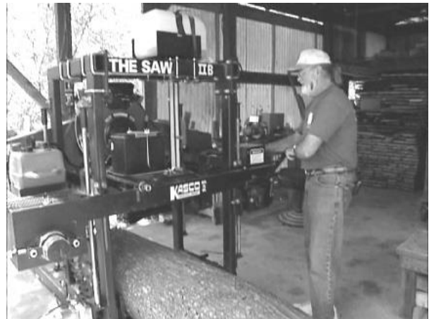
Using a band sawmill, Paul processes wood others might consider trash into value-added products on his farm.
